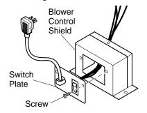
Figure 16 - Installing Switch Plate to Blower Control Shield
